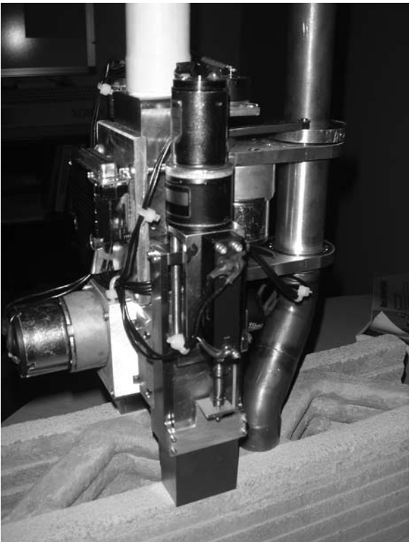
The print nozzle developed by USC’s Center for Rapid Automated Fabrication Technologies
