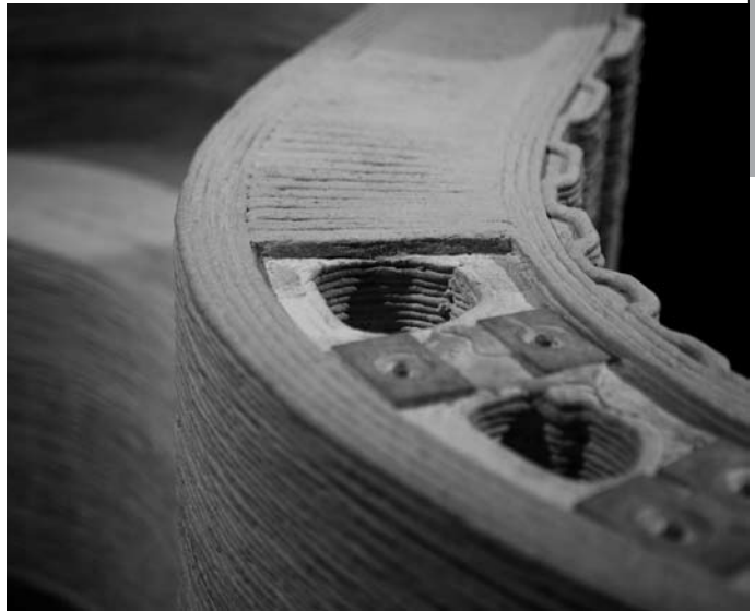
Detail of structure printed by Loughborough’s Additive Manufacturing Research Group. Photograph by Agnese Sanvito
