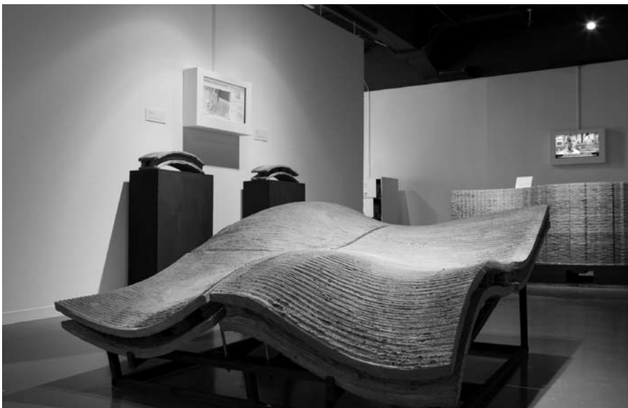
Loughborough University's Additive Manufacturing Research Group is focussing on double-curved panels for large buildings at the higher end of the market. Photograph by Agnese Sanvito
