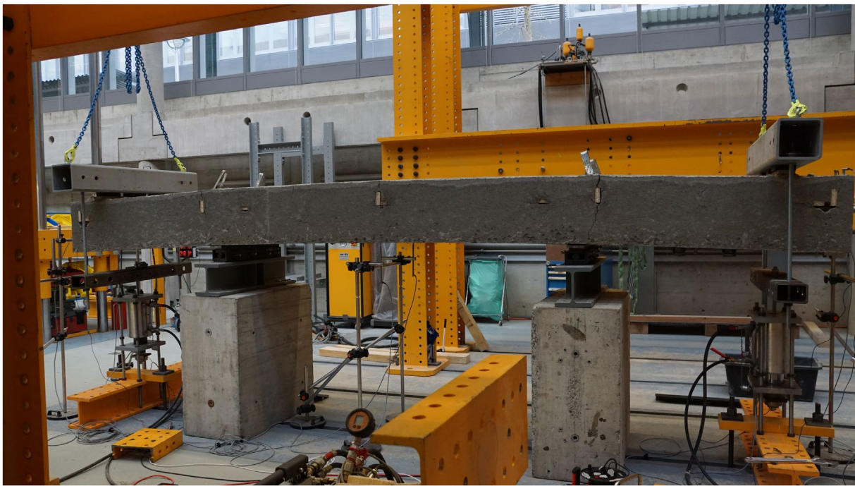
A slab of wood-based concrete undergoes stress testing at Institute for Construction and Environmental Technologies (ITEC) (credit: ITEC).
