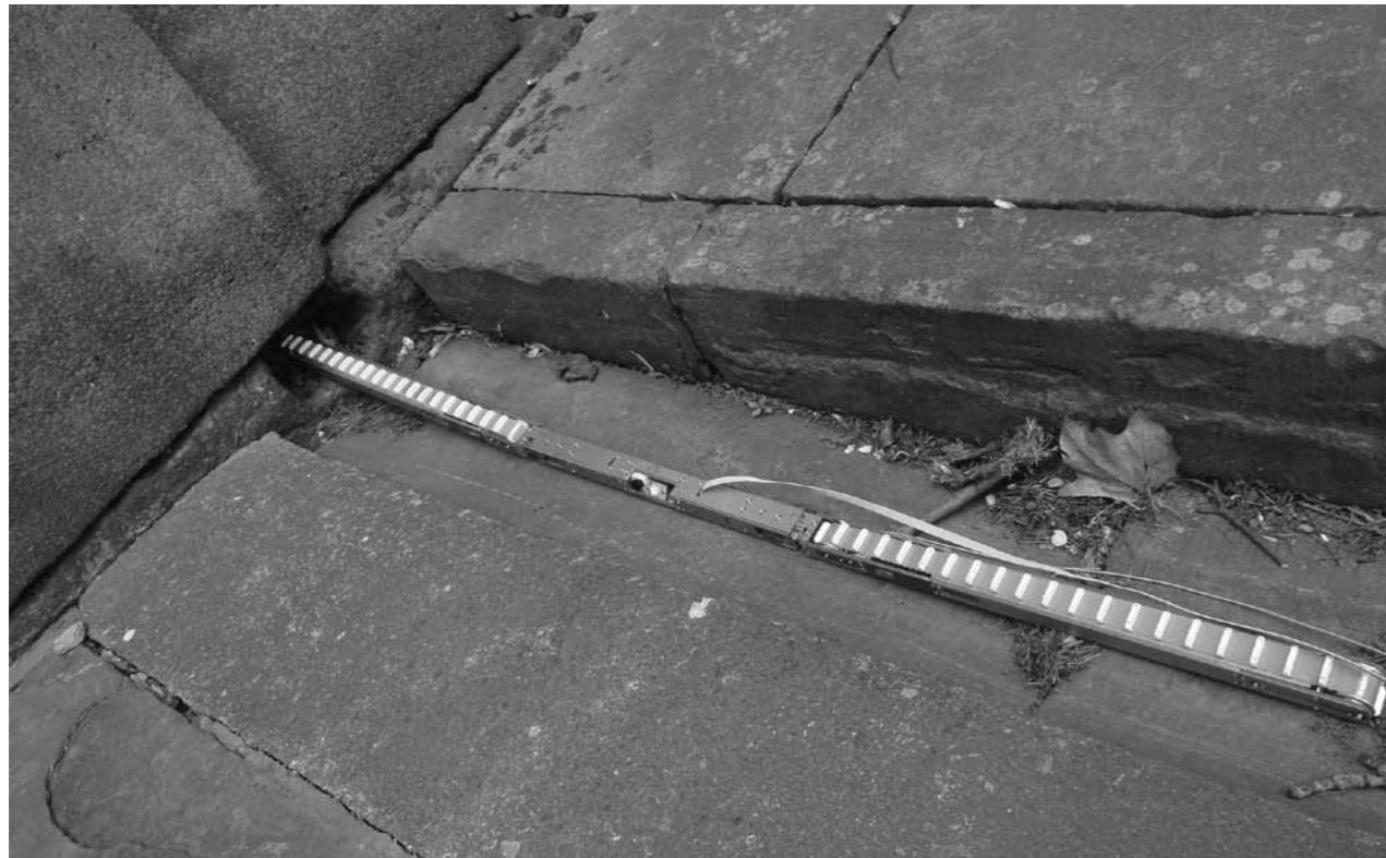
A "bore-hole deployable robot", made by the University of Leeds, can enter a 40-mm-diameter hole and then reconfigure into a U-shape for better mobility. Applications include search and inspecting disused mines
